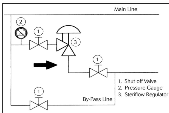
1. The valve is designed for sanitary service and it is assumed that it will be installed into a clean system. Under these conditions, special considerations to protect the valve such as providing line strainers at the valve inlet are not necessary.
