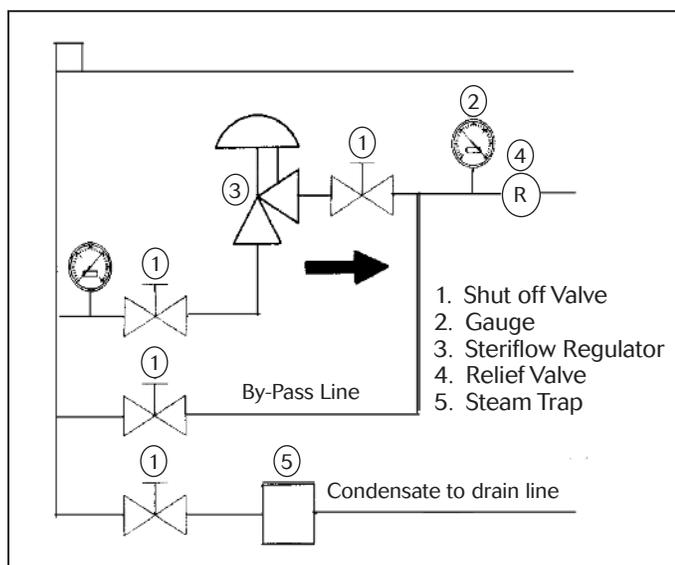
1. The valve is designed for sanitary service and it is assumed that it will be installed into a clean system. It is highly recommended that upstream lines be blown down prior to installation to remove all welding, polishing, and other debris prior to installing the valve.
